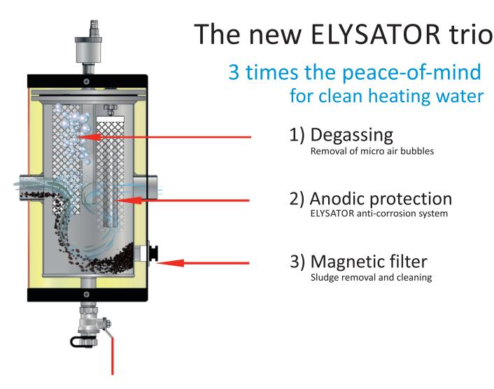
1) Degassing Removal of micro air bubbles
